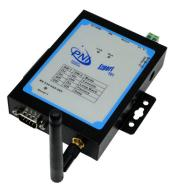
EZport provides a gateway between IP networks, ZigBee/IEEE 802.15.4 networks, and serial devices. The gateway bridges the application level data between Serial, ZigBee, and Ethernet.
